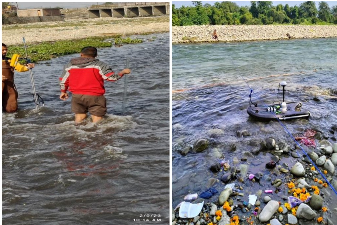
Figure 4: Discharge measurement using (A) Flow-Tracker2 in low flow condition (B) ADCP in high flow condition
